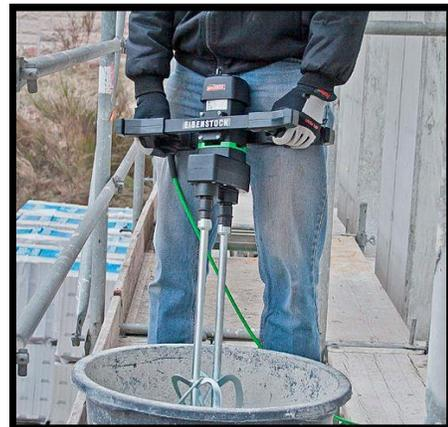
These mixers from Eibenstock are designed for mixing highly viscous and stiff materials. It has a soft start, temperature control, stepless speed regulation and constant speed. It uses two contra-rotating stirring rods and have shown that this tool cuts the mix time by half. The mixer also eliminates bucket spinning and reduces installed physical strain because of reduced torque.
